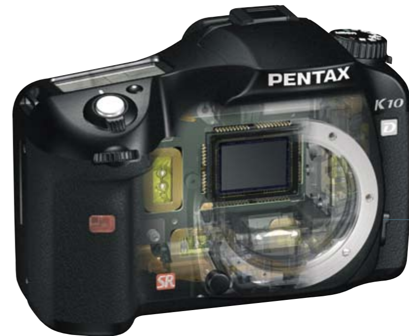
CCD plate with electromagnets to control the "Shake Reduction" mechanism is connected to permanent magnets to the metal frame as a unit.
